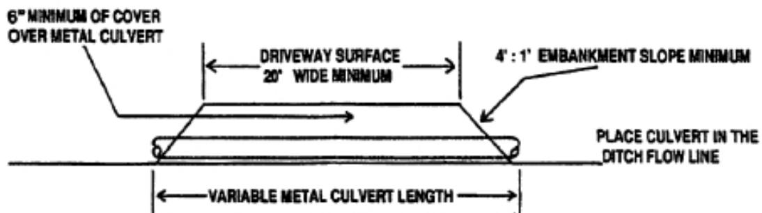
( CULVERT LENGTH DEPENDS ON THE WIDTH OF THE DRIVEWAY SURFACE AND THE DEPTH OF THE DITCH )
